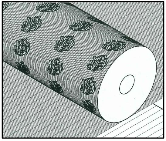
Figure 7.2.2 : Dandy Roll and Screen Error: The watermark wire forms on the dandy roll should be inverted.
